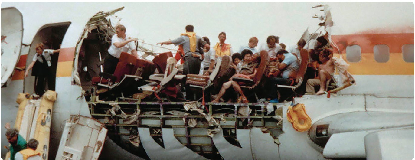
Figure 1.4 – Aloha Airlines Flight 243 – A watershed moment in aviation maintenance history that brought about much needed change in aviation maintenance. It was recognized that complacency in the state of aging aircraft was the main contributing factor to this accident.
