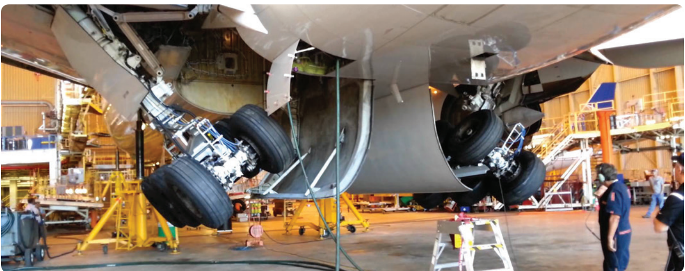
Figure 1.6 – A retraction test done after the plate was fitted as opposed to prior, would have prevented damage from this accident
