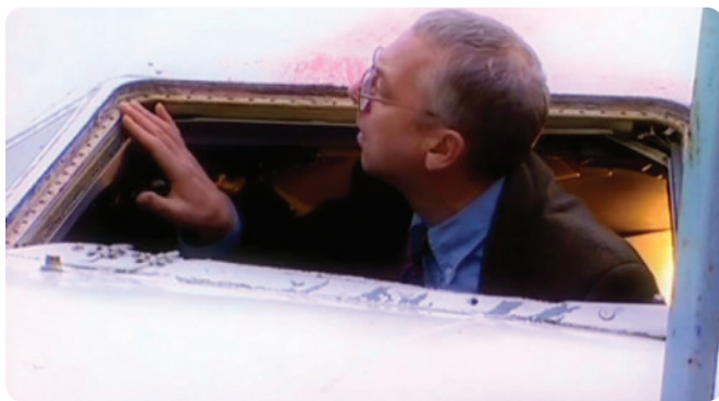
Figure 1.5 – Incorrect windscreen retention bolts; (too small) led to the windshield blowout.
